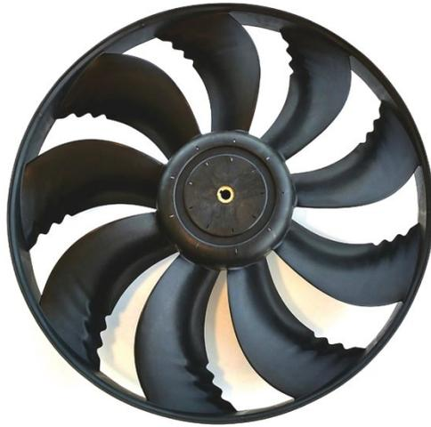
The 30KAVZE/30KAVPZE utilizes Carrier's the 6th generation Flying Bird™ fan technology, engineered for maximum efficiency, super low noise, and wide operating range. The fan includes Carrier patented rotating shroud technology and back-swept blades with a unique wave-serration trailing edge inspired from nature.
